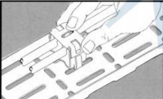
The tie bolt comes with a lock nut, ready for assembly. Put the specially designed head down through the centre hole. It will lock the clamp to the tray at the same time as the lock nut is tightened. Disassembly is done just as easily: loosen the nut and withdraw the bolt by twisting it the opposite direction.
