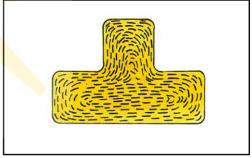
The hot forging process increases the density of the material, refines the grain structure and improves material strength.
