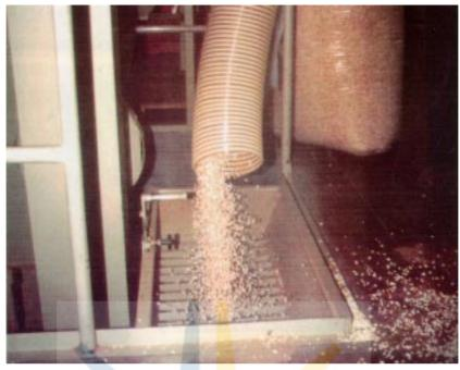
High flexibility, abrasive resistant polyurethane ducting. Ideal ducting for conveying gravel/grit/grain/corn and other dry compounds.
