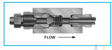
Provides unidirectional flow and tight shut off for liquids and gases with high reliability. When differential drops below cracking pressure\*, valve shuts off. (Not for use as relief valve.)
