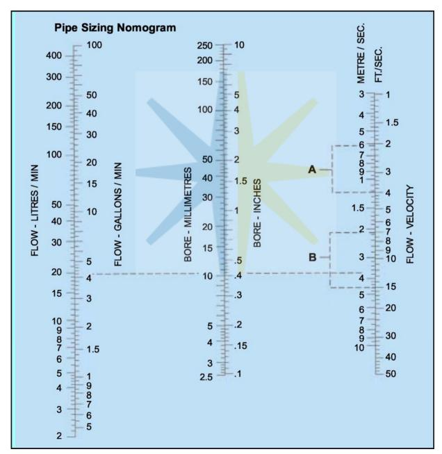
**NOTE** Flow velocities in range A recommended for return lines. Flow velocities in range B recommended for delivery lines.
